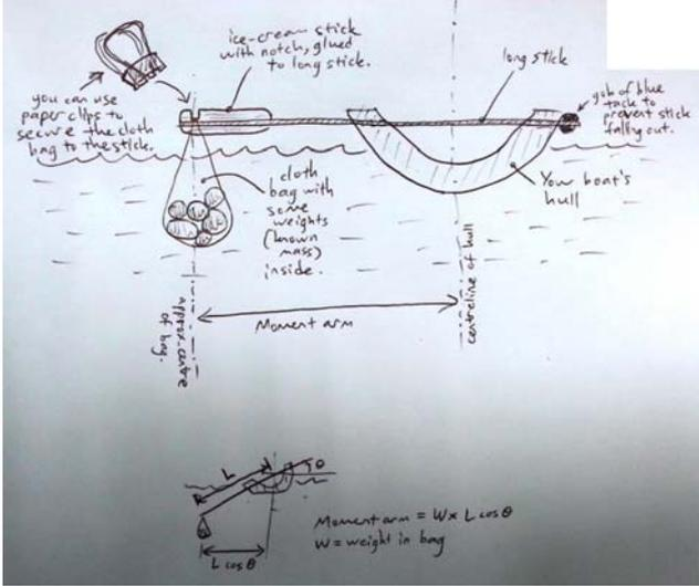
Figure 6: A simple sketch given to students to help them set up the buoyancy experiment.
