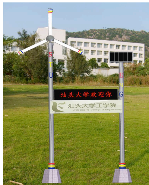
Figure 2 An Illustration of the Designed Hybrid Renewable Energy Generation Display
